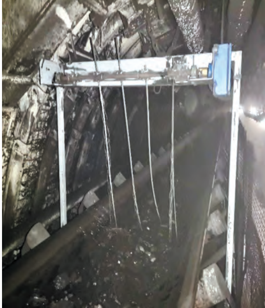
Fig. 3. Excavated material presence sensor
