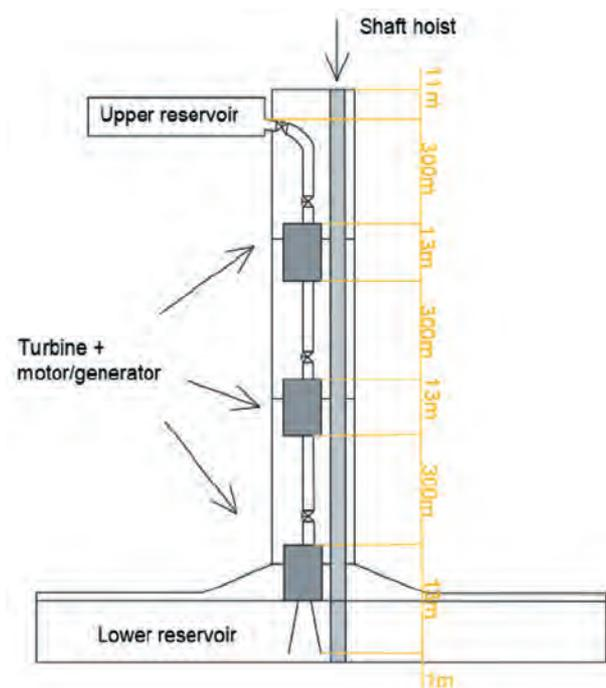
Fig. 2. UPSH infrastructure setup within the SW-3 shaft
