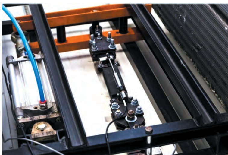
Fig. 4. Test stand for measuring the modulus of elasticity of belts in a climate chamber
