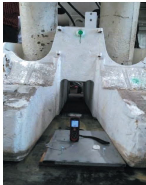
Fig. 5. Manual measurement of the powered roof support working height
